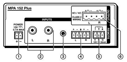
Figure 2. MPA 152 Plus Rear Panel Features
